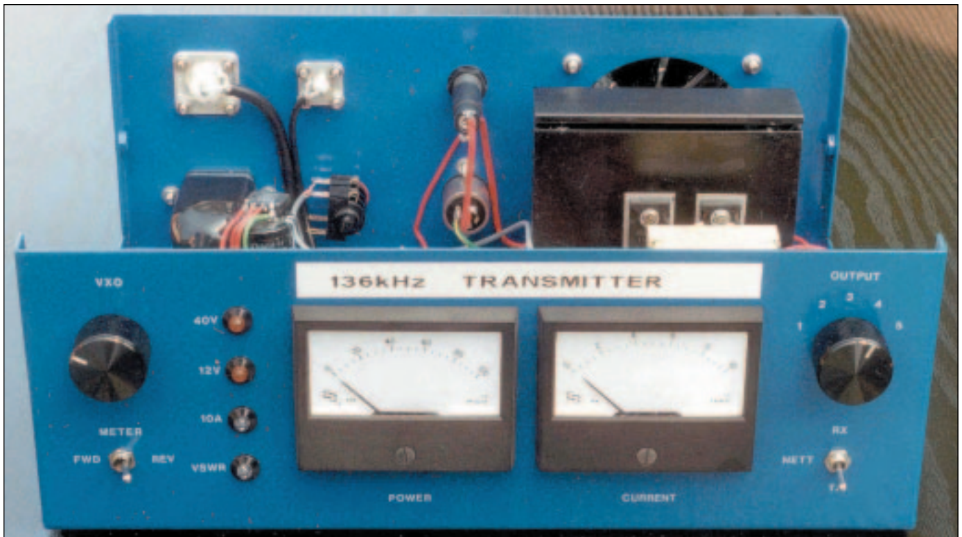
The completed 136kHz transmitter, with its cover removed.
